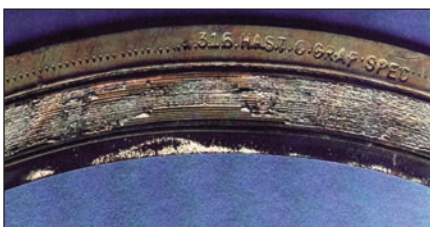
Oxidized spiral wound gasket
