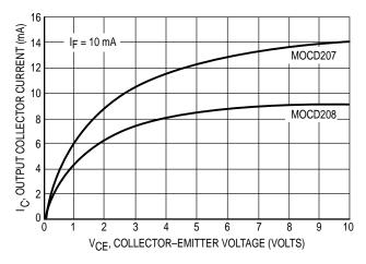
Figure 3. Output Current versus Collector–Emitter Voltage
