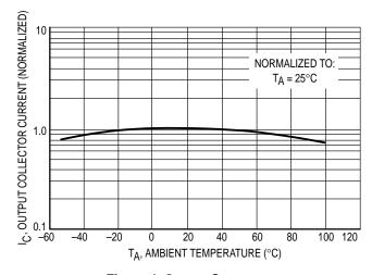
Figure 4. Output Current versus Ambient Temperature
