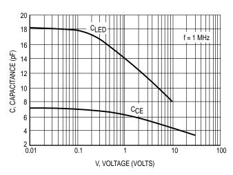
Figure 6. Capacitance versus Voltage
