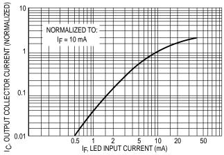
**Figure 2. Output Current versus Input Current**
