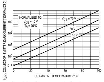
Figure 5. Dark Current versus Ambient Temperature
