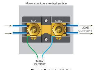
Figure 1. Typical installation
