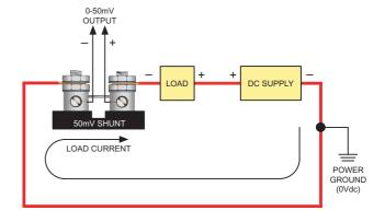
Figure 2. Typical Low-Side Shunt Connections
