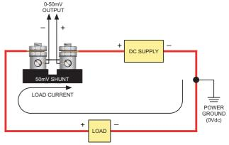
Figure 3. Typical High-Side Shunt Connections
