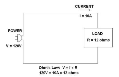
When a short circuit occurs, a low-resistive, abnormal path is created which will cause the circuit current to increase as the circuit resistance is decreased. The current when a short circuit is introduced can exceed 1000 times the normal current of the circuit. The circuit diagram of a short circuit is shown below:
