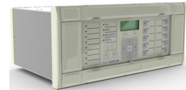
P545 Differential / Distance With Extended Binary I/O
