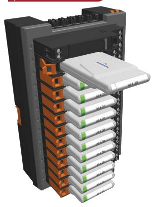
Figure 3: Each module contains HART I/O and HART digital data is extracted automatically.
