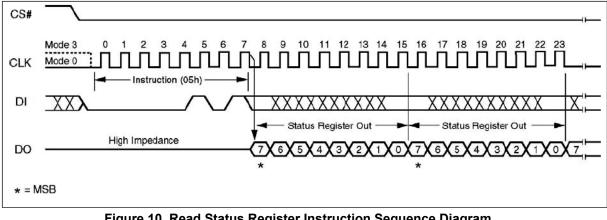
Figure 10. Read Status Register Instruction Sequence Diagram
