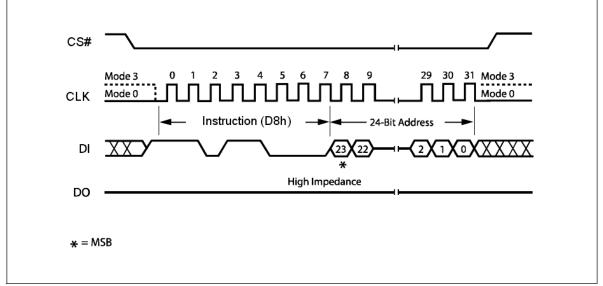
Figure 22. 64KB Block Erase Instruction Sequence Diagram
