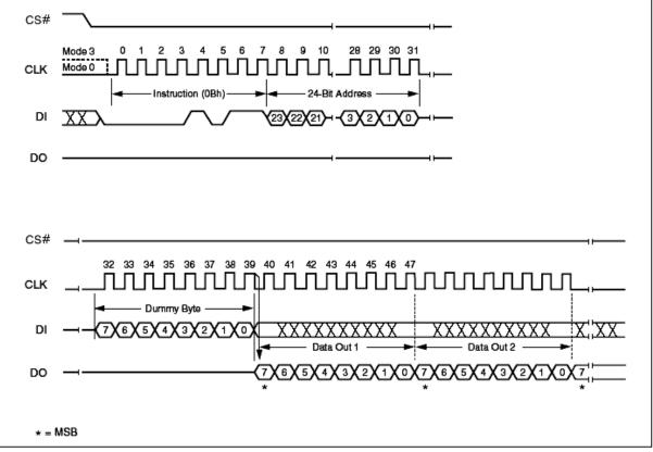
Figure 13. Fast Read Instruction Sequence Diagram
