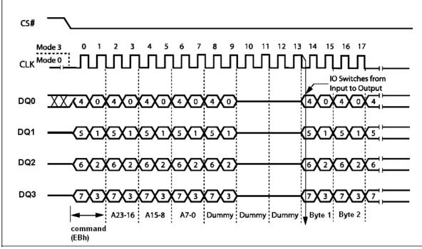
Figure 16.1. Quad Input / Output Fast Read Instruction Sequence in QPI Mode
