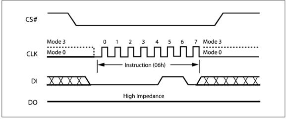
Figure 8. Write Enable Instruction Sequence Diagram
