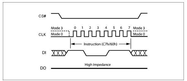
Figure 23. Chip Erase Instruction Sequence Diagram
