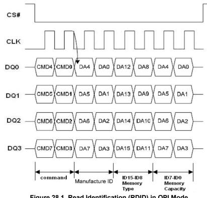
Figure 28.1. Read Identification (RDID) in QPI Mode
