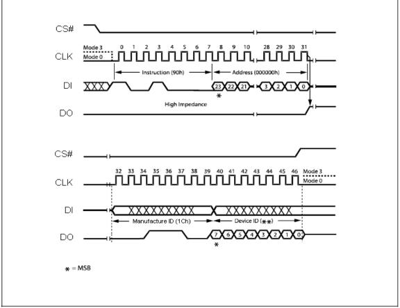
Figure 27. Read Manufacturer / Device ID Diagram
