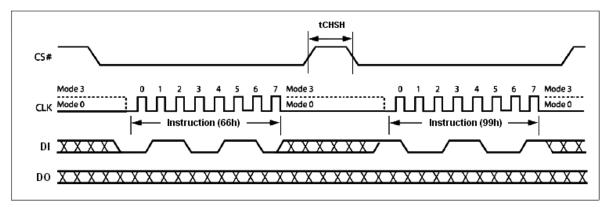
Figure 7. Reset-Enable and Reset Sequence Diagram
