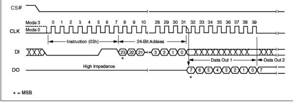
Figure 12. Read Data Instruction Sequence Diagram
