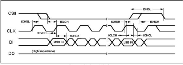
Figure 34. Input Timing
