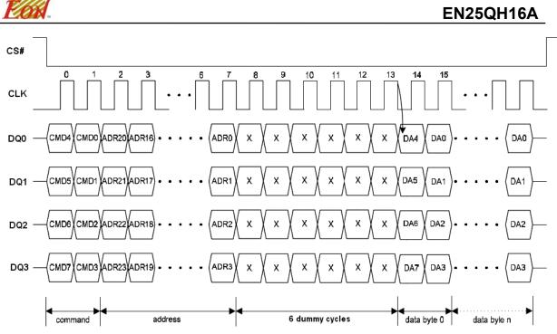
Figure 13.1 Fast Read Instruction Sequence in QPI Mode
