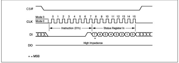
Figure 11. Write Status Register Instruction Sequence Diagram
