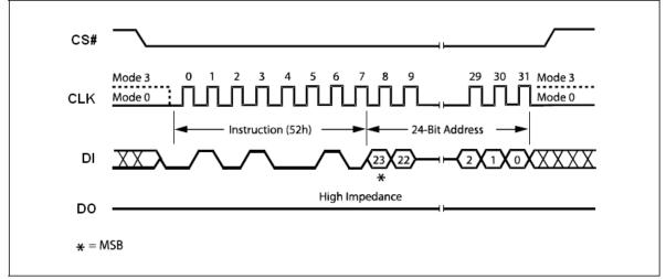
Figure 21. 32KB Half Block Erase Instruction Sequence Diagram
