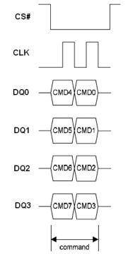
Figure 23.1 Chip Erase Sequence in QPI Mode
