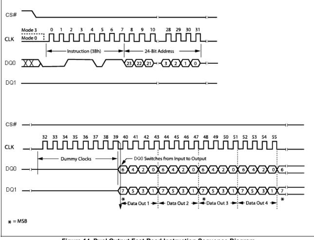
Figure 14. Dual Output Fast Read Instruction Sequence Diagram
