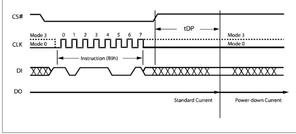
Figure 24. Deep Power-down Instruction Sequence Diagram
