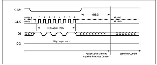
Figure 25. Release Power-down Instruction Sequence Diagram
