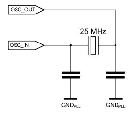
Figure 42: Quartz crystal connection
