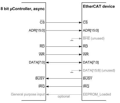
Figure 23: Connection with 8 bit µControllers (BHE and DATA[15:8] should not be left open)
