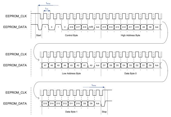
Figure 40: Write access (2 address bytes, 32 kBit - 4 MBit EEPROMs)
