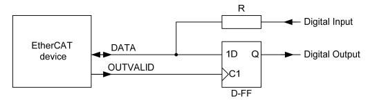
Figure 10: Bidirectional mode: Input/Output connection (R=4.7kΩ recommended)
