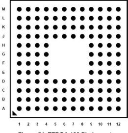
Figure 54: TFBGA 128 Pin Layout
