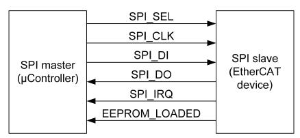
Figure 15: SPI master and slave interconnection
