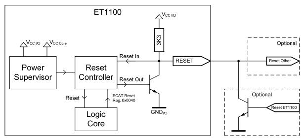
Figure 50: Reset Logic
