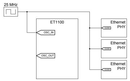
Figure 44: Oscillator clock source for ET1100 and Ethernet PHYs
