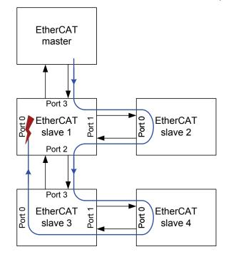
Figure 7: All frames are dropped because of Circulating Frame Prevention
