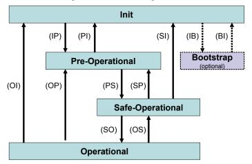
Figure 36: EtherCAT State Machine
