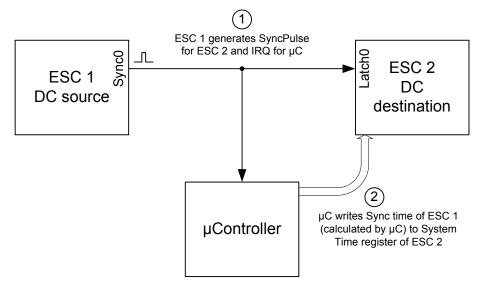
Figure 34: System Time PDI Controlled with two steps
