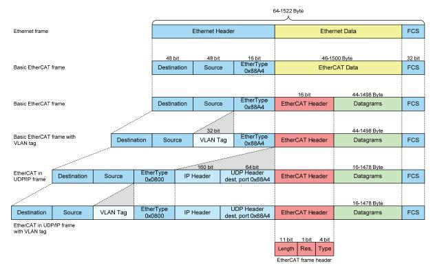
Figure 2: Ethernet Frame with EtherCAT Data
