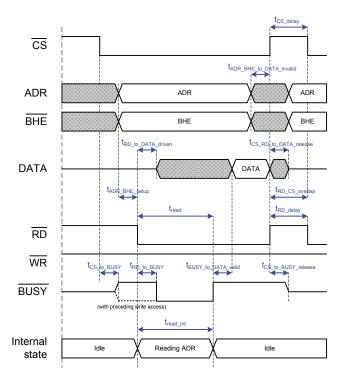
Figure 24: Read access (without preceding write access)
