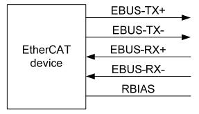
Figure 17: EBUS Interface Signals
