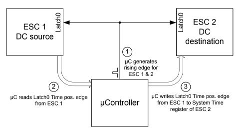
Figure 33: System Time PDI Controlled with three steps
