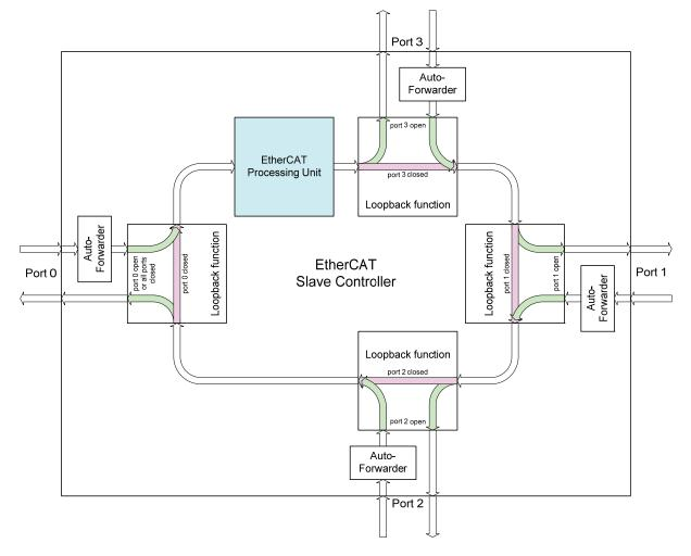
Figure 5: Frame Processing
