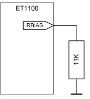
Figure 49: LVDS load resistor
