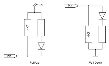
Figure 46: Dual purpose configuration input/LED output pins
