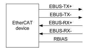
Figure 7: EBUS Interface Signals
