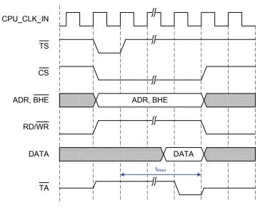
Figure 35: Read access (CS together wit TS, CS and TA on rising edge)
