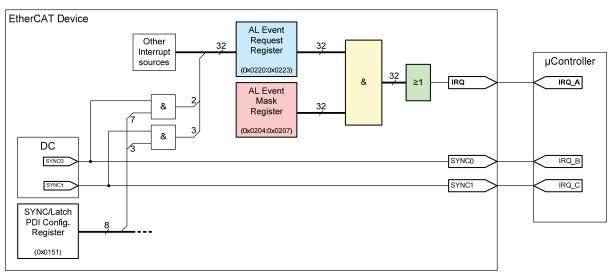
Figure 42: PDI Interrupt Masking and interrupt signals
