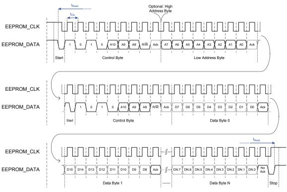
Figure 41: Read access (1 address byte, up to 16 kBit EEPROMs)
