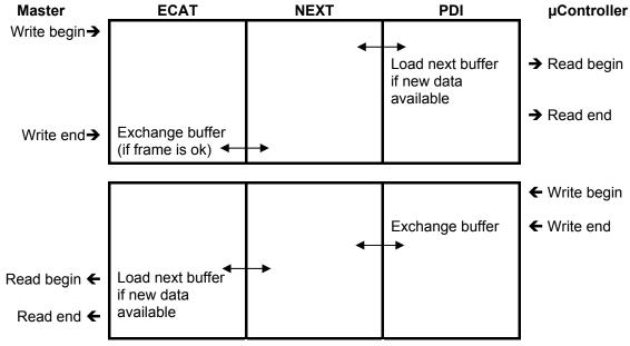
Figure 24: SyncManager Buffered Mode Interaction
