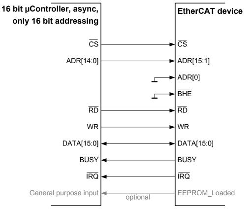
Figure 22: Connection with 16 bit µControllers without byte addressing
