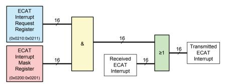
Figure 43: ECAT Interrupt Masking
