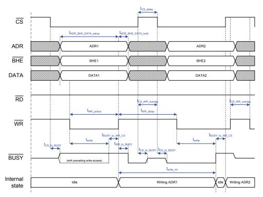
Figure 25: Write access (write after rising edge nWR, without preceding write access)
