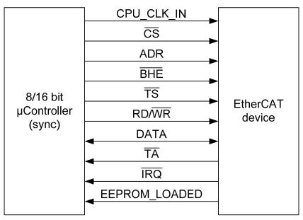
Figure 27: µController interconnection<sup>4</sup>
