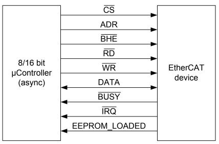
Figure 21: µController interconnection<sup>3</sup>
