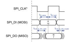
Figure 16: Basic SPI\_DI/SPI\_DO timing (\*refer to timing diagram for relevant edges of SPI\_CLK)
