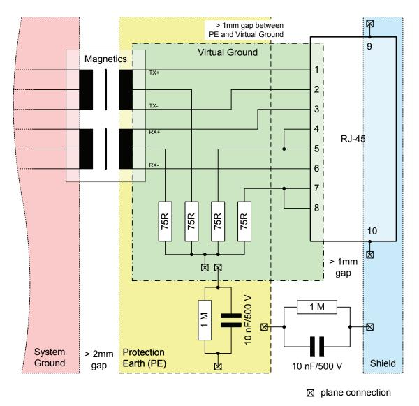
Figure 12: Termination and Grounding Recommendation
