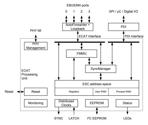
Figure 1: ET1100 Block Diagram
