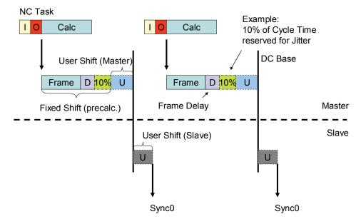
Figure 35: DC Timing Signals in relation to Communication
