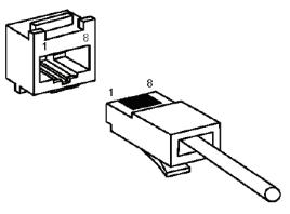
Figure 13: RJ45 Connector
