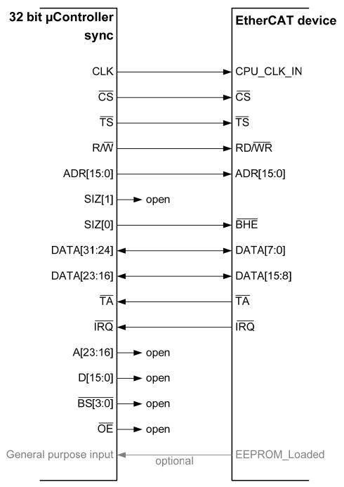
Figure 30: Synchronous 32 bit µController connection using Transfer Size
