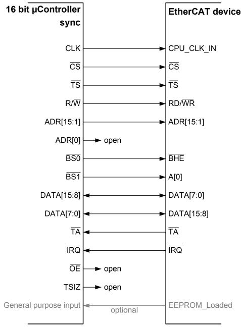
Figure 29: Synchronous 16 bit µController connection using Byte Select
