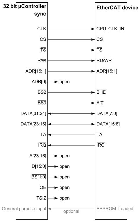
Figure 28: Synchronous 32 bit µController connection using Byte Select
