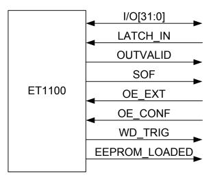
Figure 8: ET1100 Digital I/O signals
