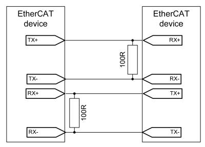
Figure 20: EBUS Connection
