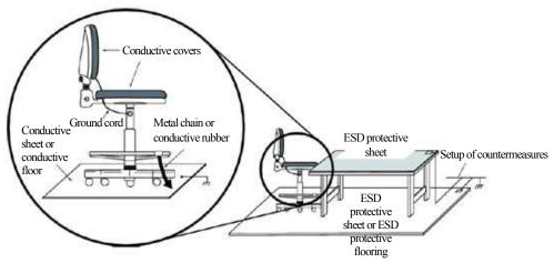
Figure 37 – Example of countermeasures for workbenches and work area
