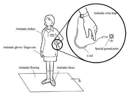
Figure 39 - Example of countermeasures used by worker
