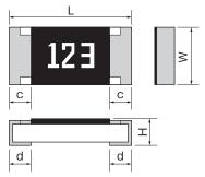
Rated resisitance value is marked with 3-digit (E24) on the over coating except 4-digit (E96).
