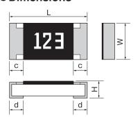
Rated resistance value marking is with 3-digit (E24) or 4-digit (E96) on the over coating except RMGW10. 4-digit marking is available for F tolerance except RMGW16 & RMGW10.
