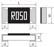
Rated resistance is marked with 4-digit on the over coating. (RLC20~RLC63) RLC10 : only No marking is available.
