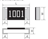
Rated resistance value is marked with 3-digit (E24) or 4-digit (E96) on the over coating. RNC06: only No marking is available.
