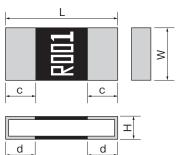
Resistance value of RLP series are marked like below. The resistance value of RLP63 & MLP63 are marked with 4 characters on the overcoating. The resistance value of RLP20 & RLP32 are marked with "2 numbers" & "\_" on the overcoating.
