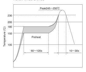
2. Flow soldering (Recommended condition of Sn solder and Sn-Pb solder)
