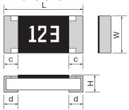
Rated resistance value marking is on the over coating except RMNW10 & RMAW10.
