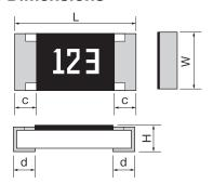
Rated resistance is marked with 3-digit (E24) or 4-digit (E96) on the over coating. RVC16 : only 3-digit marking is available.
