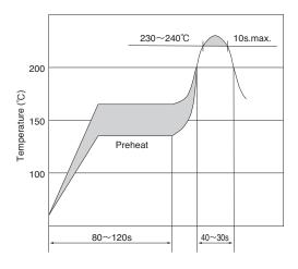
1.2 Recommended condition of Sn solder Reflow times: 2 times
