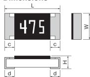
Rated resistace is marked with 3-digit(E24) on the over coating.
