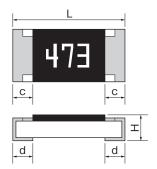
Rated resistance value marking is with 3-digit (E24) or 4-digit (E96) on the over coating. RGC1/16: only 3-digit marking is available.
