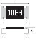
Rated resistance and T.C.R. value are marked with 4-digit on the over coating.
