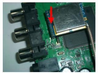
2: Putting the module on the carrier board with socket.
