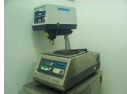
TOOL : POLISHING MACHINE BRAND/MODEL : BUEHLER/ECOMET 3 APPLICATION : CROSS SECTION
