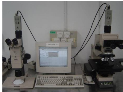
TOOL : POWER SCOPE BRAND/MODEL : OLYMPUS APPLICATION : VISUAL INSPECTION
