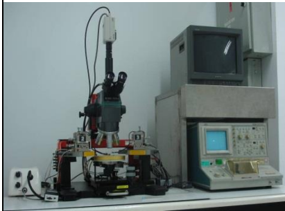
TOOL : PROBE STATION BRAND/MODEL : SINGATON / S-1170 APPLICATION : PROBE DIE
