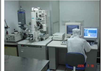
TOOL : SEM / EDX BRAND/MODEL : HITACHI/S-4700 OXFORD/7200 APPLICATION : MICROSTRUCTURE OBSERVATION
