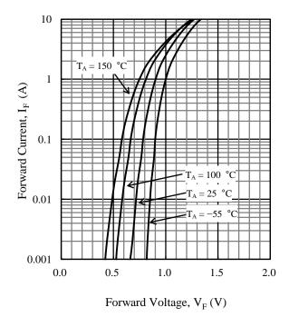
Figure 19. SJPZ-N33 Typical Characteristics: V<sub>F</sub> vs. I<sub>F</sub>
