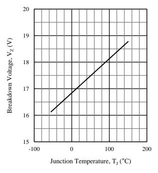
Figure 8. SJPZ-N18 Typical Characteristics:  $V_Z$  vs.  $T_J$
