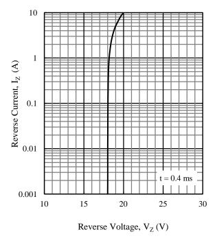
Figure 7. SJPZ-N18 Typical Characteristics: I<sub>Z</sub> vs. V<sub>Z</sub>
