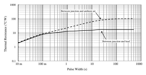
Figure 18. SJPZ-N33 Typical Transient Thermal Resistance<sup>(12)</sup>
