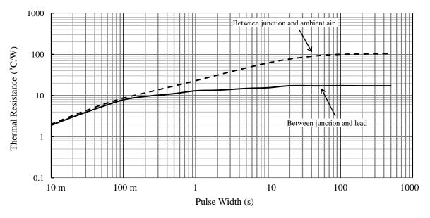
Figure 11. SJPZ-N27 Typical Transient Thermal Resistance<sup>(9)</sup>
