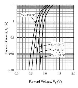
Figure 5. SJPZ-N18 Typical Characteristics:  $I_F$  vs.  $V_F$
