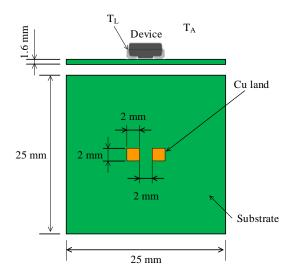
Figure 1. Lead Temperature Measurement Conditions
