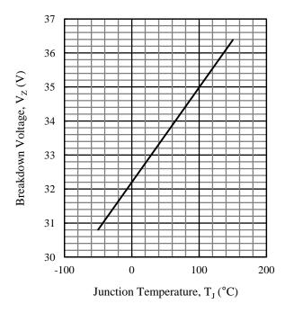
Figure 22. SJPZ-N33 Typical Characteristics:  $V_Z$  vs.  $T_J$
