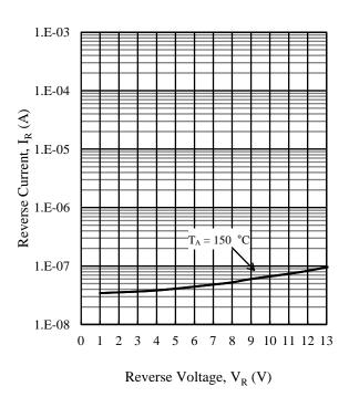
Figure 6. SJPZ-N18 Typical Characteristics: I<sub>R</sub> vs. V<sub>R</sub>
