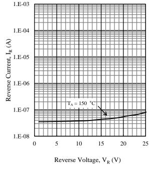
Figure 20. SJPZ-N33 Typical Characteristics:  $V_R$  vs.  $I_R$
