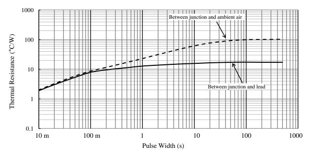
Figure 4. SJPZ-N18 Typical Transient Thermal Resistance<sup>(6)</sup>
