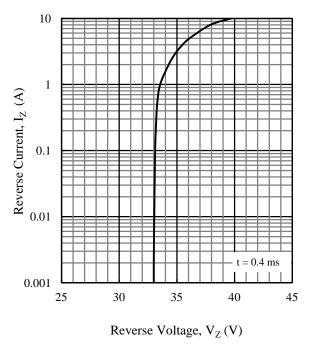
Figure 21. SJPZ-N33 Typical Characteristics:  $I_Z$  vs.  $V_Z$
