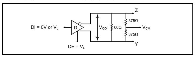
FIGURE 7. RS-485/422 DRIVER OUTPUT SHORT CIRCUIT CURRENT
