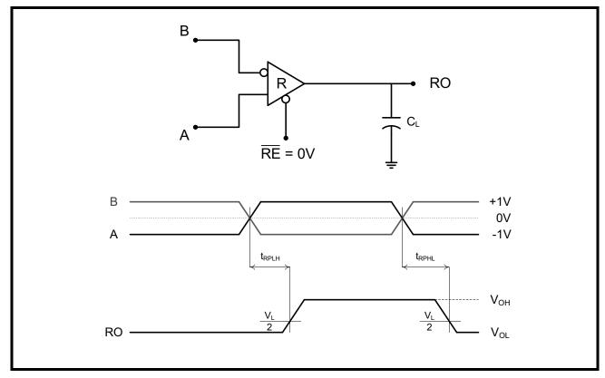
FIGURE 11. RS-485/422 DRIVER PROPAGATION DELAY AND RISE/FALL TIMES
