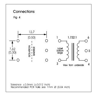
Dimensions shown are in millimetres (inches). Geometric centres of outline and pin grid coincide within a tolerance circle of 0.6mm
