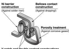
V notch and Double contact constructions (Against foreign particles and flux!)
