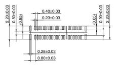
Recommended metal mask pattern Metal mask thickness: When 120μm (Terminal opening ratio: 70%)
