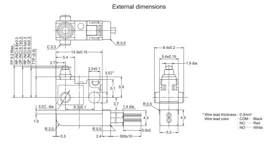
Wire leads left side type: Mounting hole 3 mm, standard type
