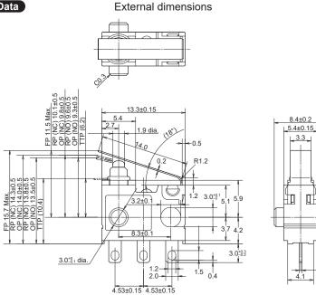
Note: When switching at high speed or under shock, lever endurance may drop. Therefore, please be sure to conduct an endurance evaluation under actual switching conditions. (Unit: mm) General tolerance: ±0.25
