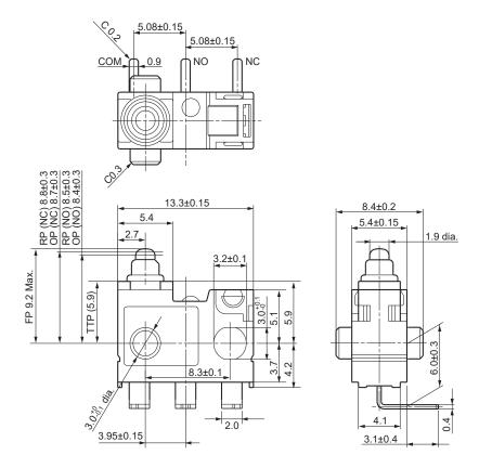
Angle terminal type: Mounting hole 3 mm, standard type (Left type)
