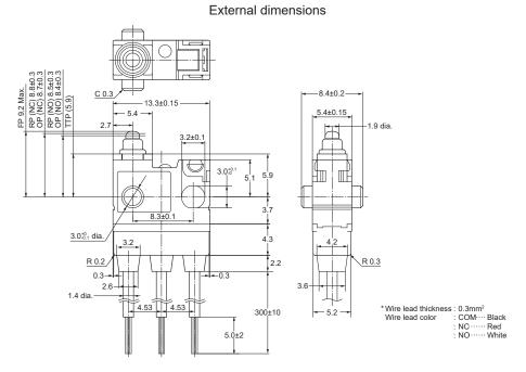
Wire leads right side type: Mounting hole 3 mm, standard type
