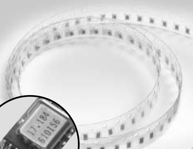
Typical installation in TCXO (temperature compensated crystal oscillator) application
