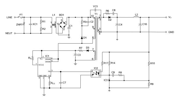
Fig.8 UTC UCS16505S Typical Application Circuit
