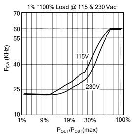
Fig.4 The relation curve between f<sub>SW</sub> and relative output power P<sub>OUT</sub> / P<sub>OUT (MAX)</sub>
