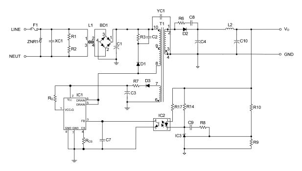
Fig.7 UTC UCS1652S Typical Application Circuit
