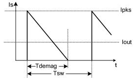
Figure 4. Secondary current waveform
