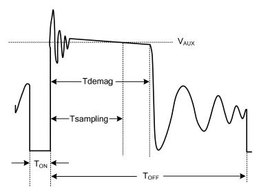
Figure 2. Auxiliary voltage waveform
