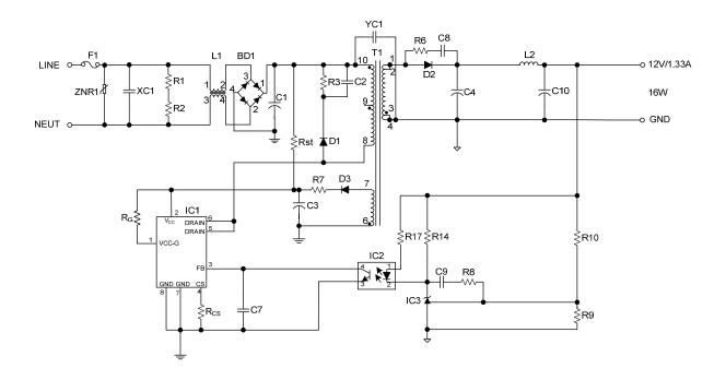
Fig.10 UTC US1602 Typical Application Circuit
