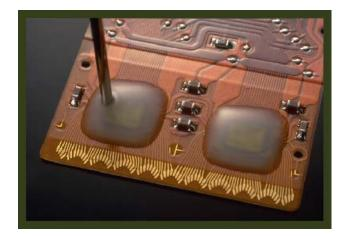
Photo: UVE-1017-2 on a polyimide flexible circuit.
