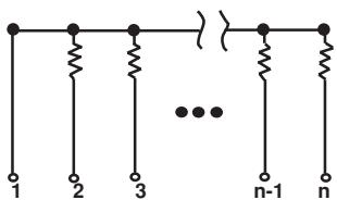
5, 7 or 9 resistors with one pin common
