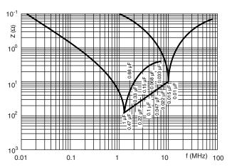
Impedance (Z) as a function of frequency (f) at  $T_a = 20\,^{\circ}\text{C}$  (average) Measurement with length 6 mm
