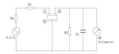
R1=280 Ω  $\pm$ 5%,R2=330Ω $\pm$ 5%,Rg=50Ω ①:Input
