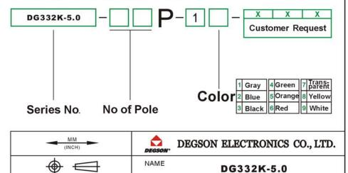
DG332K-5.0 is a 5.0mm Plug from Degson that is compatible with a Pin-Strip, it is a very competitive Plug & Socket combination. The plugs are interlocking so can be made up with any number of ways and the Pin-Strip comes in a 24 way as standard but are easily snap-able down to any number of ways.
