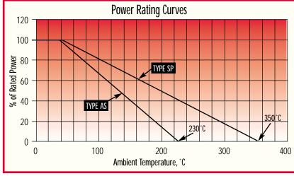
Power ratings are based on maximum allowable surface temperature in still air at  $40^{\circ}\text{C}$  ambient temperature.
