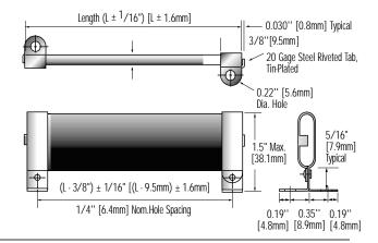
Figure 5. With Low Profile Axial Tabs (H1)
