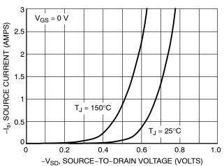
Figure 10. Diode Forward Voltage versus Current
