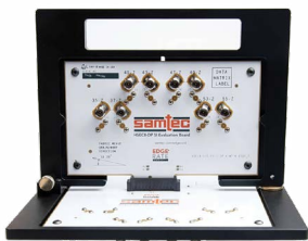
Generate™ Differential Pair Edge Card (HSEC8-DP) REF-210637-X.XX-XX
