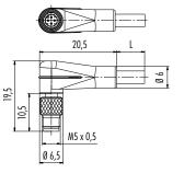
Female cable connector, moulded, M5 x 0,5/moulded, shielded, M5 x 0,5
