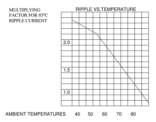
Ripple current capability depends upon case area and ESR because ripple current dissipates power in the ESR and case area determines the core temperature rise. A different capacitance from that listed in Standard Ratings Table will have a different ESR and, therefore, a different ripple current rating. The ripple capability is proportional to square root of capacitance for the same WVdc and case size.
