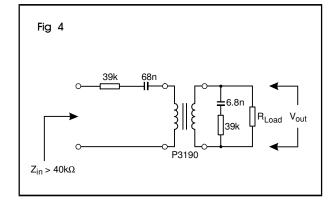
Due to the finite primary inductance of the P3190, the circuit of Fig. 3 suffers from low frequency rolloff below 500Hz. At the expense of around 6dBV loss, the circuit of Fig. 4 provides a relatively flat response from 300Hz to 4kHz.
