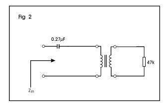
In practice, the  $47k\Omega$  load can be increased without limit. The DC blocking capacitor should be maintained within the range  $0.22\mu F$  to  $0.33\mu F$  to obtain a flat frequency response and input impedance to specification.
