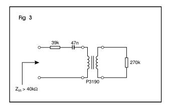
At the expense of a small loss, the circuit in Fig. 3 provides an impedance exceeding  $40 k\Omega$  from DC upwards.
