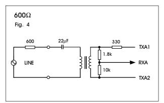
Frequency Response : ±0.1dB 30Hz – 10kHz Return Loss: 25dB 200Hz – 4kHz Transhybrid Loss: 18dB 200Hz – 4kHz
