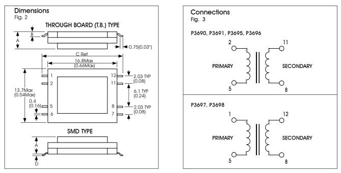
Dimensions shown are in millimetres (inches). Windings may be used interchangeably as primary or secondary.
