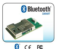
The **PAN1721** is an ideal choice for applications where battery life is a critical application requirement, using only 500 nA in sleep mode. Short transition times between operating modes—3 uS Wake-Up – and power efficient hardware further reduce current consumption.
