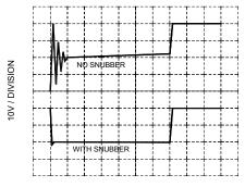
FIGURE 2: WAVEFORM WITH AND WITHOUT SNUBBER
