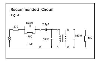
In practice, the  $600\Omega$  load resistor will connect to a low output impedance TX driver. The 150nF capacitor should appear in parallel with the  $680\Omega$  load resistor (rather than in parallel with transformer winding) to obtain optimum TX flatness to line.
