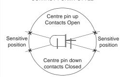
Contact Form/Style: Switch types CW1600 may have a normally open or closed contact depending on the positioning of the switch. These switches have a change in sensitivity depending on the switch position.
