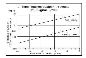
Third order intermodulation products 2fa-fb and 2fb-fa are of most importance and are significantly greater than products 2fa+fb and 2fb+fa. Figure 8 gives the total power of all distortion products within the voiceband.
