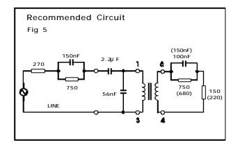
Figure 5 gives flat RX and TX responses against the reference impedance (typically around  $\pm 0.5$ dB 300Hz - 3.4kHz). Return loss is typically better than 20dB. The circuit values in parentheses give optimum flatness at a small sacrifice in return loss.
