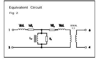
Typical lumped parameters as Fig. 2, referred to pins 1-3.
