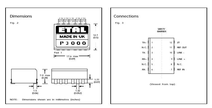
Geometric centres of outline and pin grid coincide within a tolerance circle of 0.6mmØ.
