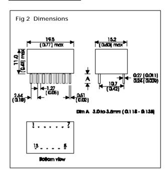
Dimensions are in millimetres (inches) - not to scale.
